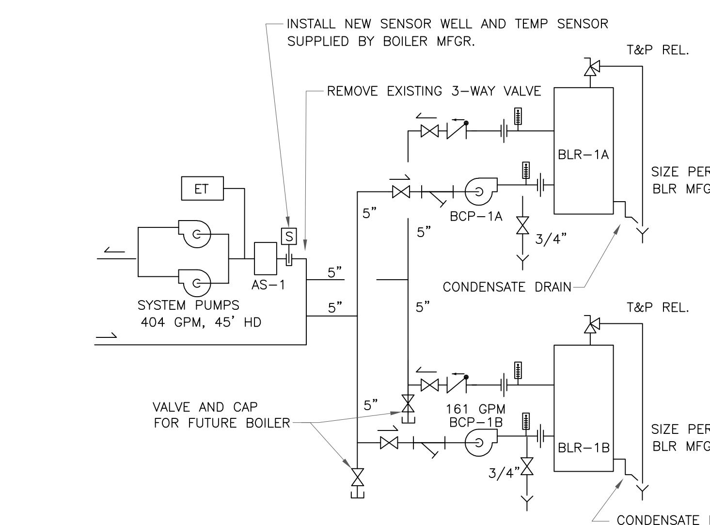
C NEW BOILERS PIPING SCHEMATIC
